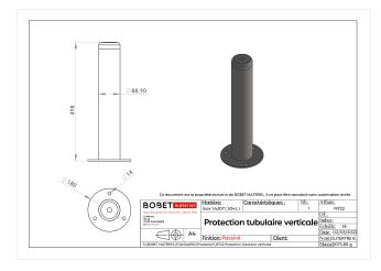
This tubular protection offers a barrier of protection against shocks caused by the traffic of pallet trucks, forklifts, etc.
