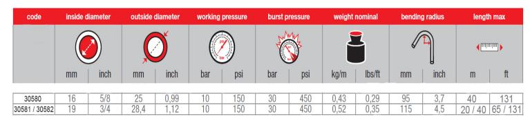
Hose for washing with hot water in the food industry, with very good resistance to high temperatures. Ideal for all washing and cleaning operations in dairies, canneries, slaughterhouses and food industries. Extremely grease resistant coating. Not suitable for transporting food
