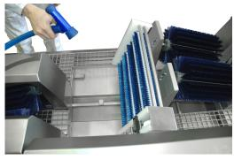
The Compact Corridor CC2002 provides cleaning and disinfection for boots, shoes or clogs with smooth personnel flow at the beginning or the end of the day work (two-way traffic possible). It can be fitted as a "compulsory walk-through" before access to production areas or cloakrooms.
